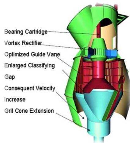
**Figure 11 New Classifier with vortex rectifier**
