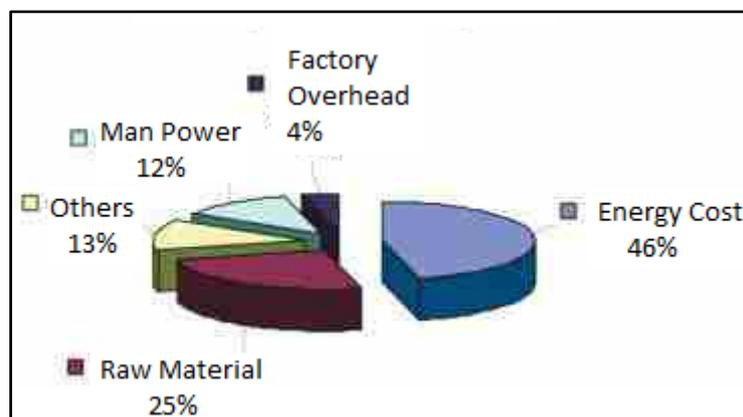
**Figure 5 Break-up of Cement Manufacturing Costs**
