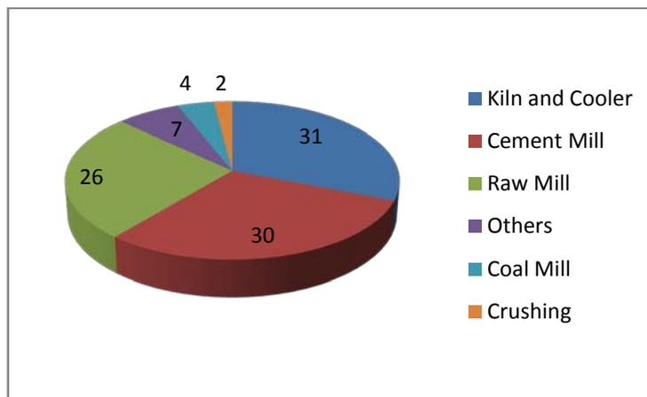
**Figure 6 Break-up of Electrical Energy Consumption**
