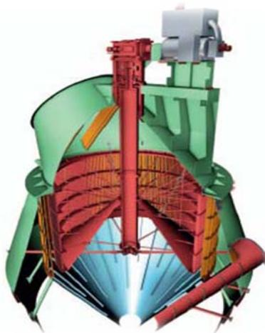
**Figure 12 Old Classifier without vortex rectifier**
