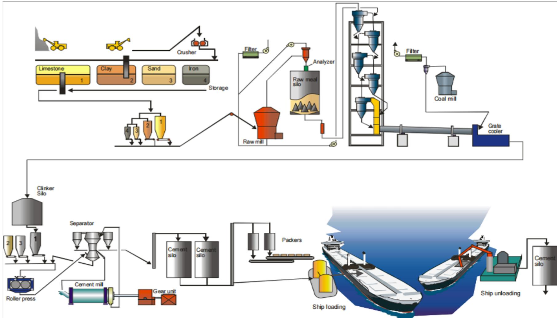
Figure 7 Process flow sheet of a typical Cement Plant
