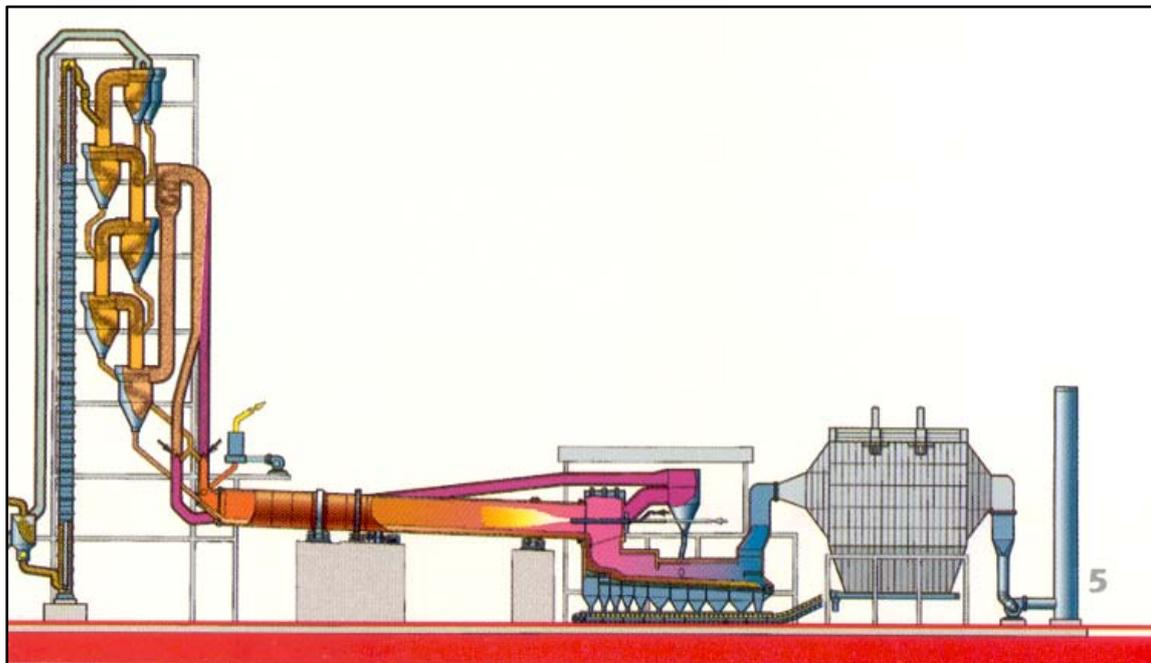
**Figure 9 Pre-heater, Pre-Calciner, Kiln and Cooler System**
