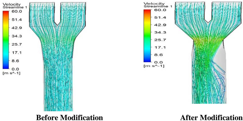
**Figure 18 Line-2 Cement Mill bag house fan outlet duct:**
