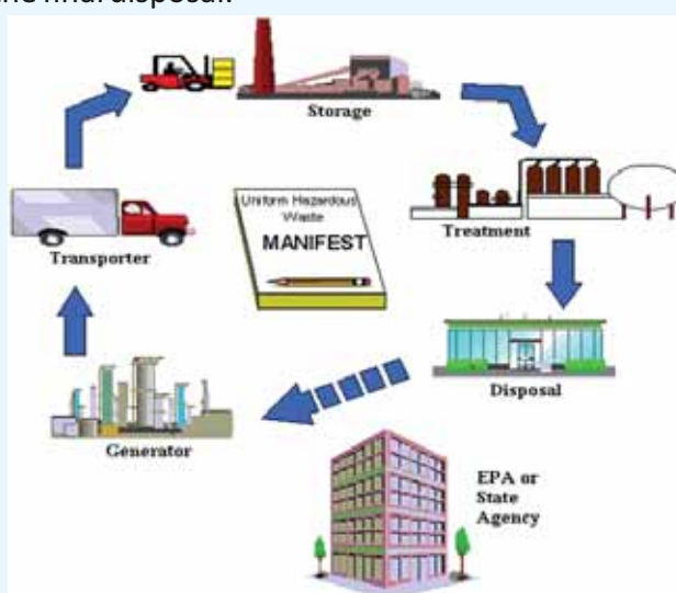
Figure – 7.2.1: Showing pathway of hazardous waste movement
