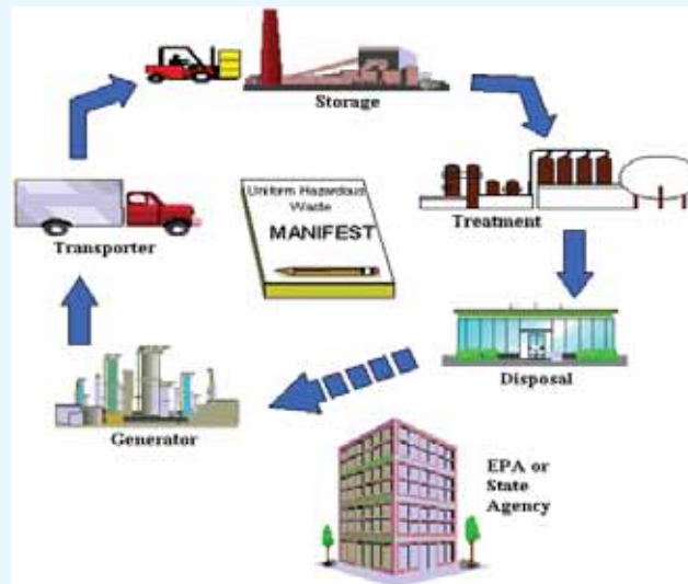
Figure - 1: Showing pathway of hazardous waste movement
