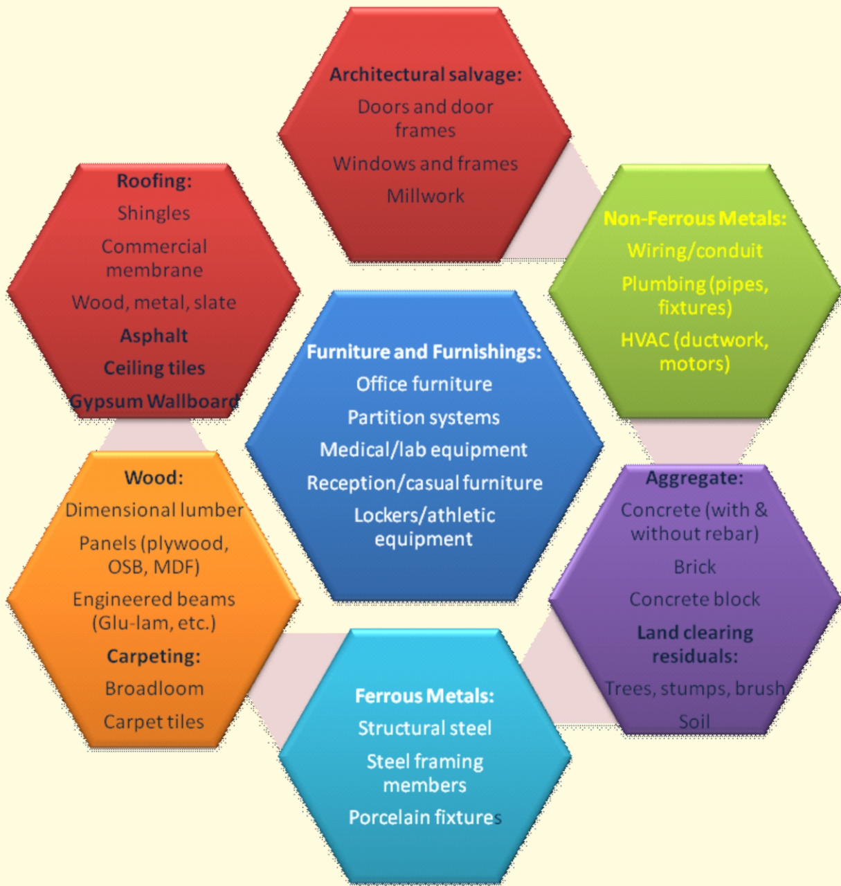
Figure 4.3 – Physical Composition of C&D Waste
